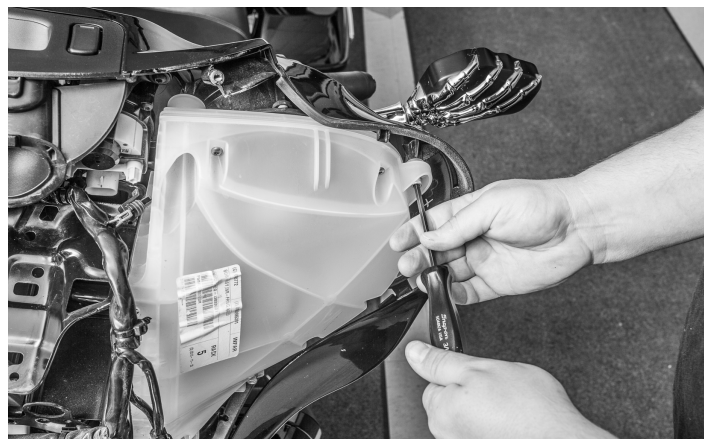
Next, remove the last three screws that hold the pod to the fairing.
