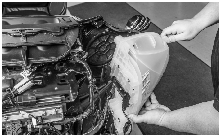
Remove the fairing and set aside for the speaker removal.
