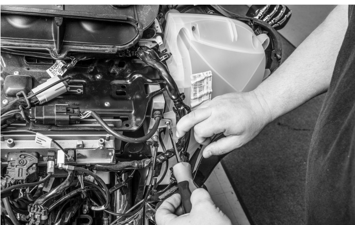
If your bike is equipped with the optional communication setup, you will need to remove the module to access mounting bolts.
